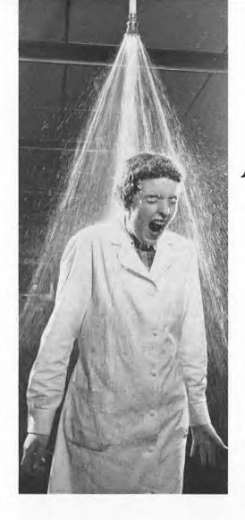
DRENCHING spray water will smother burning clothing or still the savage eating of full-strength acid. That's why a special shower head hanging from the ceiling is a necessary part of the safety equipment in Parker Pen's chemistry laboratory. A flick of a nearby quick-action valve produces the pictured results. Lab assistant
